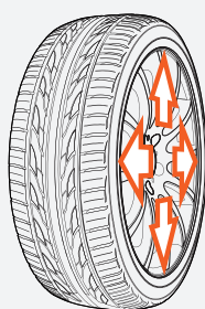
Rim clamping from inside
