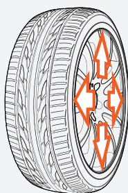
Rim clamping from inside
