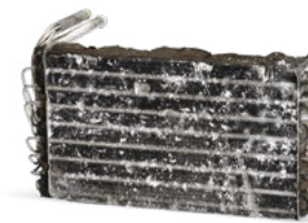
Without A/C maintenance
